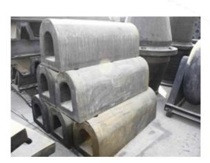
Rubber D fenders provide an excellent barrier protection for port sides, vessels, trucks and loading bays. They are used to absorb the kinetic energy of a boat or vessel berthing against a jetty, quay wall or other vessel to prevent damage.
